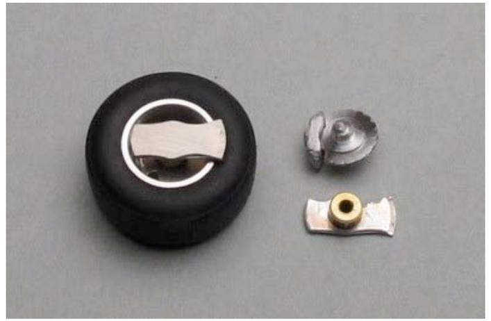
I temporarily built the inner unit of the front wheel and checked its depth. It seems better to reduce the thickness of the brake disk half as I had given a moderate curve to the wheel spoke.
