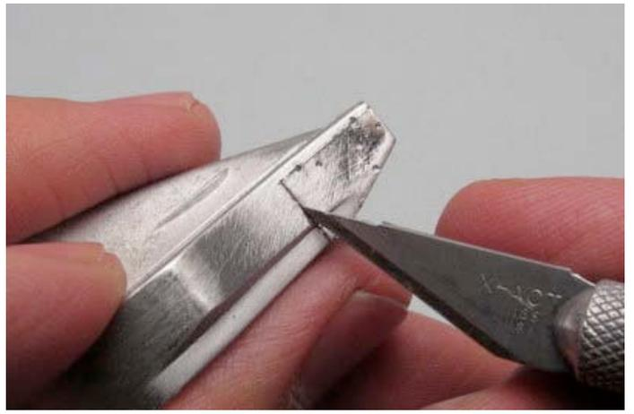
Around the rear suspension panel, I used this Xacto knife. It makes engraving straight lines easy.
