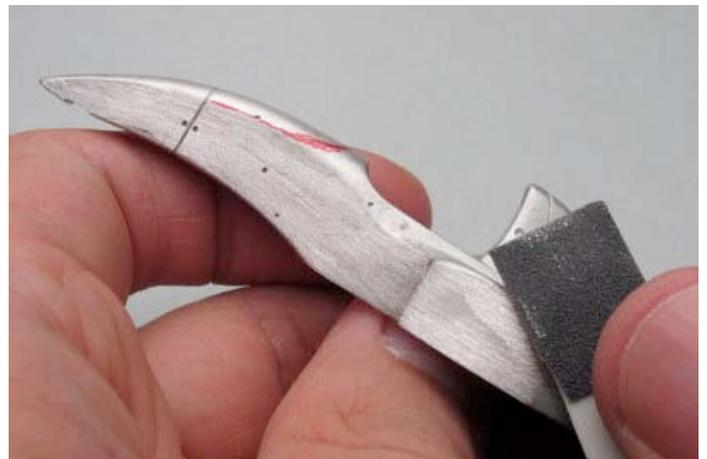
The clean main body castings were welcome but I had to sand a few parting lines on the side. The styrene plate backing is necessary to make a sharply chiseled face in such an instance.
