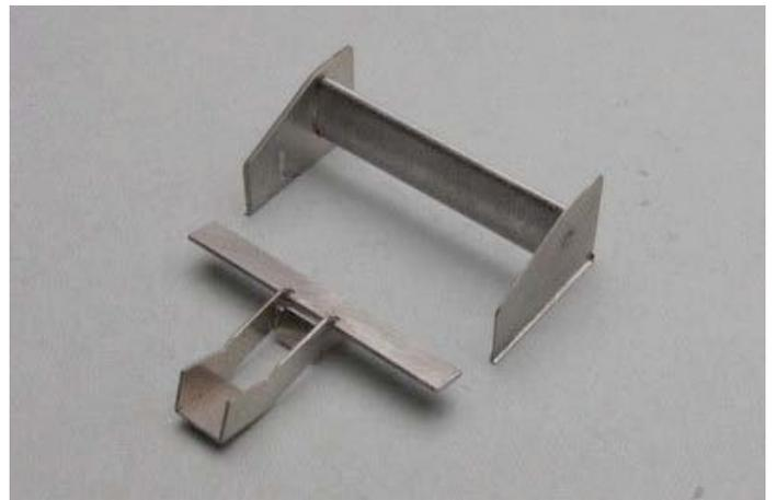
I joined the main wing and the end plates with solder. The mount and the lower part of the wing will be attached after painting.
