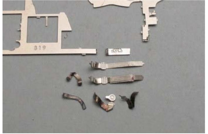
I formed PE seat belt parts after annealing with burner. The both sholder pads came from PE sprue and I soldered them on the belt back.
