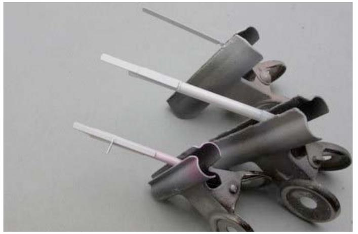
These flaps look difficult to hold for painting. I usually leave PE sprues intact for easier clamping, however, this time I had to cut them off for the test-fitting with the end plates. So this combination of double-faced tape and styrene rod was the alternative.
