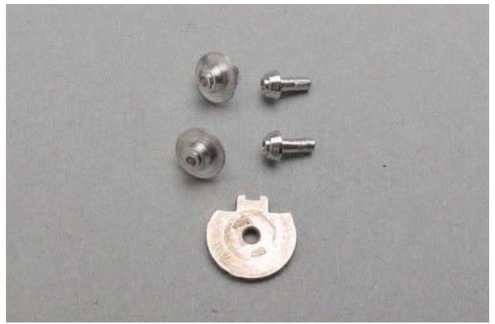
Then I removed the axle pieces from the brake disc and reduced their depth with motor tool to narrow the front tread
