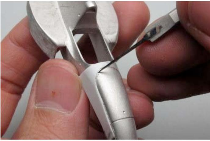
First I made a jig with a thin styrene sheet and then engraved a line along it with a micro chisel, little by little
