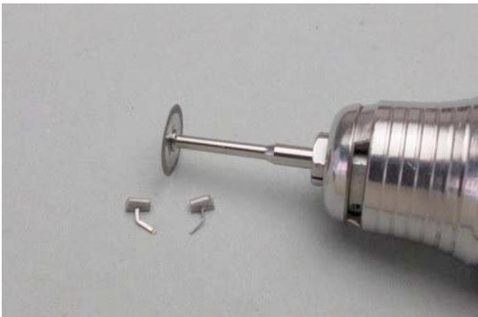
The original PE mirror stem looks too thick... I reduced its diameter with a moto tool after I joined it to the bottom of mirror.
