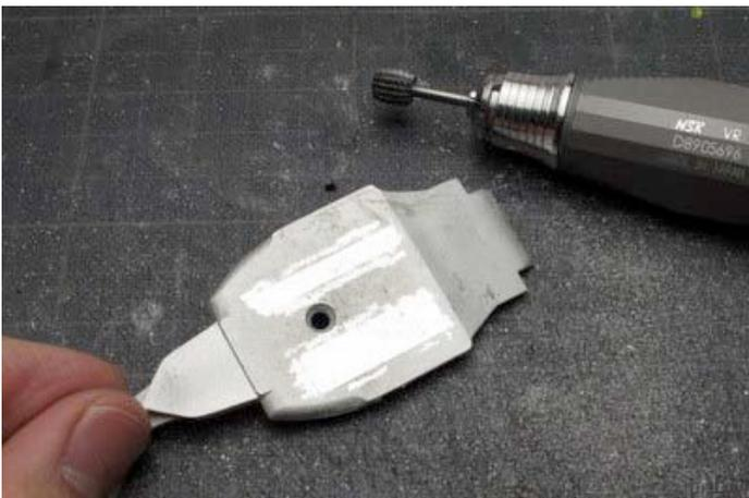
Unfortunately I had to remove the original Tameo Kits engraving on the base plate to set the ride-height accurately.
