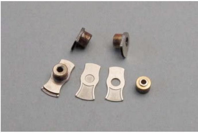
The brake ducts were assembled with solder. I use low temperature solder which fuses around 165 degrees centigrade and low-power iron -15 wattage.
