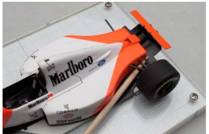
I began the suspension assembly after I finished the sensitive adjustment of the front wing flap. The tooth pick was keeping the position of the push rod until the adhesive dries.
