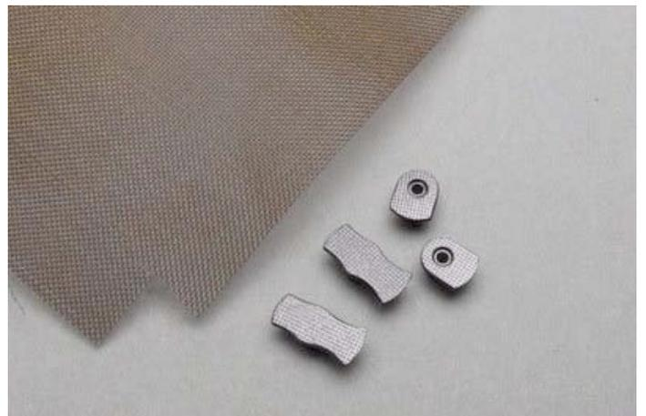
I painted brake ducts black and decorated them with carbon fiber pattern. It was very easy work with a micro mesh close to the black surface, and then I over-sprayed silver paint lightly.
