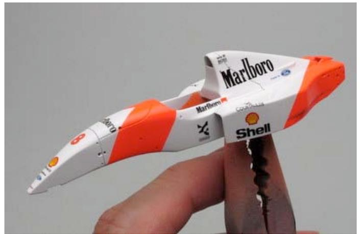
I started the clear coating process. Never spray thick coat on the decals at the first layer. Unfortunately, some dust and lint were caught on the surface of the third layer. I just stopped my airbrush and waited until the layer had dried enough until I could sand to remove them
