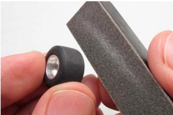
I sanded the tires smooth with #320-400 sandpaper, and then made a flat spot on the bottom.
