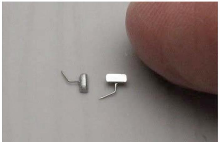
Then I modified the shape of the outer cases and polished the face of each mirror with a lapping film.
