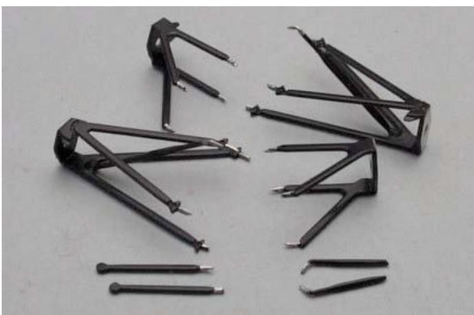
The suspension arms were painted black, too. Better to peel off the paint around the base of the parts to attach them to the body more easily.
