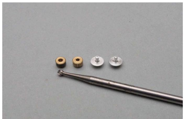
In terms of the center pieces of the axle, there were some burrs which interfere with smooth assembly. I removed them by hand with this round cutter.
