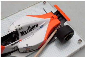
I began the suspension assembly after I finished the sensitive adjustment of the front wing flap. The tooth pick was keeping the position of the push rod until the adhesive dries.
