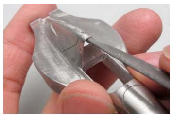
Trimming around the edges of the air intake required a sensitive touch.
