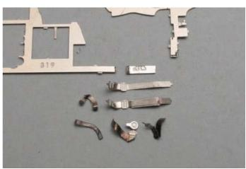
I formed PE seat belt parts after annealing with burner. The both sholder pads came from PE sprue and I soldered them on the belt back.
