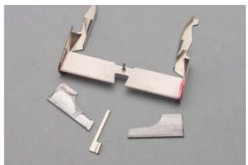
Something strange occurred when I preassembled the wing unit. I modified valley foldlines on the both flaps with solder and sanded them smooth with a gentle curve. I also attached a chip of PE sprue at the inner-end of the flap to extend it.
