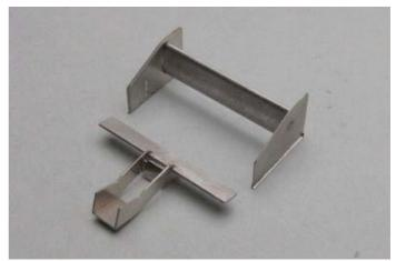
I joined the main wing and the end plates with solder. The mount and the lower part of the wing will be attached after painting.
