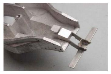
A test-fitting of the rear wing unit to the body showed me that I have to raise the mount up about 2mm. I removed the thickness of the mount block and raised its height... it took a bit of finesse.
