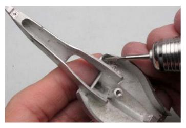
I removed the front edges of each side pod. If you want to open the air intake, the moto tool is a big help to when removing a lot of metal.
