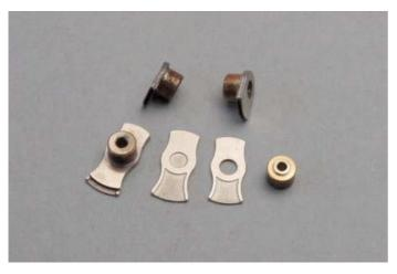
The brake ducts were assembled with solder. I use low temperature solder which fuses around 165 degrees centigrade and low-power iron -15 wattage.
