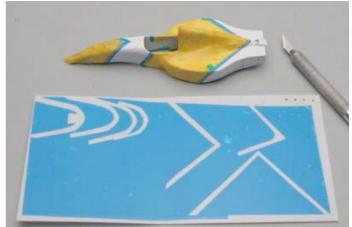
I tried to apply the orange decals but I couldn't manage it. So I changed plans and began to mask the body for two tone painting instead. The blue material is a pressure-sensitive adhesive masking sheet for airbrush artwork which I bought at an art supply store.
