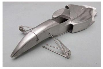
I tried to fit the arms to the body, however, it needed relocation of the attachment holes to get the correct position.
