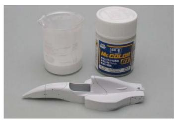
It was time to paint the body white. I put 7ml thinner into a glass beaker and made a 10ml mixture of white lacquer paint which can be passed through Tamiya's 0.2mm diameter air brush. Then I sprayed it carefully about 5 or 6 times.
