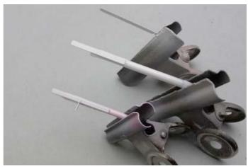
These flaps look difficult to hold for painting. I usually leave PE sprues intact for easier clamping, however, this time I had to cut them off for the test-fitting with the end plates. So this combination of double-faced tape and styrene rod was the alternative.
