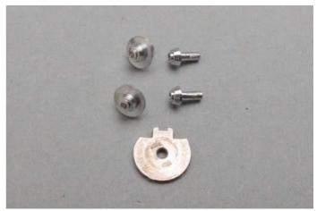
Then I removed the axle pieces from the brake disc and reduced their depth with motor tool to narrow the front tread
