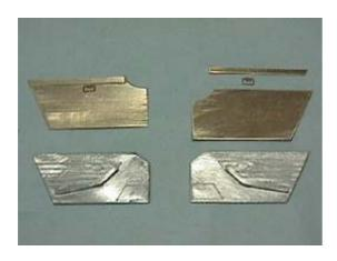
I made the interior trim for the front doors. The trim included in the kit was for the road cars. The interior panels in the Daytona Group 4 were simpler, so I cut 0.5-mm brass and nickel silver plates to make a new pair. I made the handle with a photo-etched part from a 1/35th tank kit.
