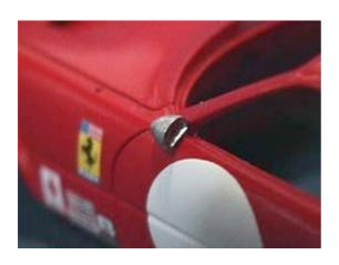
I used Tron's detail part for the left side rearview mirror. I drilled it a 0.5 mm hole, and inserted a nickel silver rod. I drilled a 0.6 mm hole in the body, and I will attach the mirror in the end.
