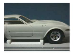
I pre-assembled the body and the chassis, and then put them on the jig I made with a 1.0-mm styrene plate and a 0.5-mm rod.
