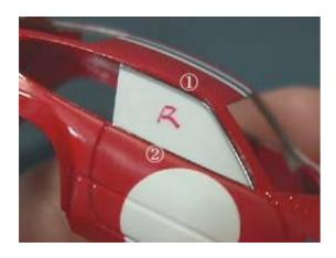
Then, I made the main side window frames. The top frame was made with the 0.5-mm strip (Number 1) and the bottom frame was with the 0.3-mm strip (Number 2), and I polished them with #2000 sandpaper and the rubber polishing burr on the rotary tool. I glued them with super glue.
