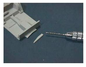
The chassis cracked when I put a tip of the drill on the chassis without any pressure. Scary!
