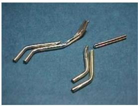
I inserted the 1.6-mm brass rod inside the brass tube. I heated them well, and put them on the vise. I shaped them by bending with force.
