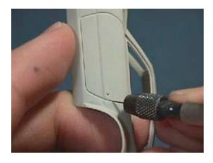
On the main body, the recessed lines were well molded, so I only deepened them with a fine needle.
