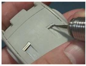
I did the same to the air outlet on the hood. I glued a strip of 0.2-mm nickel silver plate with super glue and I filled a gap with a minimal amount of epoxy filler.
