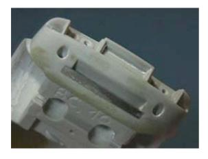
There is an air intake on the nose, and so I replaced the lip with a 0.2-mm nickel silver plate.
