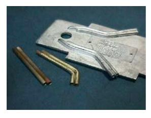
I hadn't made the exhaust pipes yet. I used a 1.8-mm brass tube and a 1.0-mm brass rod.
