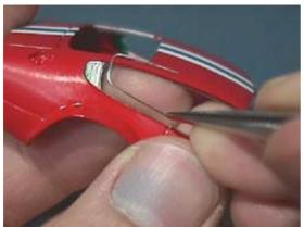
I bent the rod to shape the frame, and then polished it. Unlike the front door window frame, I will glue this in the end.
