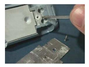
I joined the body and the underbody tray with a screw. Since I cannot put the screw into the resin, I applied epoxy filler around it
