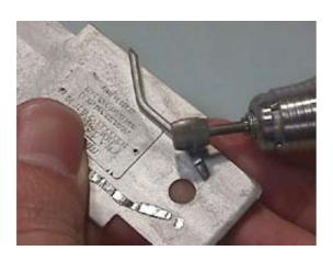
An exhaust pipe was molded on the chassis on each side, but there should be two pipes on each side. I deleted the moldings.
