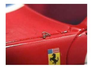
I made the base for the catch pin with a brass rod.
