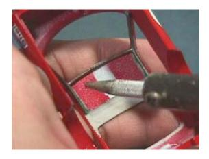
The front half of the roll cage was made with a combination of 1.2-mm nickel silver rod. I measured the length of the A-pillar and cut the nickel silver rods. Then, I soldered them to the body.
