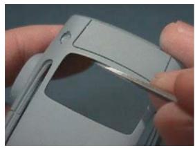
It is crucial that the opening be adjusted perfectly. If I file too much, there will be a gap between the body and the fame. If I don't file enough, the edge of the opening will be visible through the window. Mind you, we're talking about a margin of 1mm!
