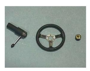
I painted the steering wheel rim semi matt black. The steering wheel shaft was made with a combination of brass tubes.
