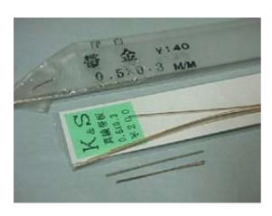
As I wrote on March 30, the frame for the side window was too small. I remade it with the nickel silver strip.
