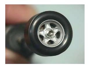
After the glue hardened, I attached the center lock. The disk brake rotor is visible through the wheel as you can see in the picture.
