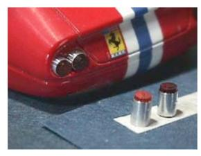
The brake lamps were machined with a 3-mm aluminum tube, and the colored acrylic tubes.
