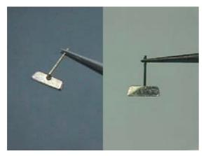
The rear view mirror was made with a nickel silver plate. I polished the part, and then soldered a 0.3-mm rod. I painted the whole thing black, and then peel the paint to expose a mirror surface.
