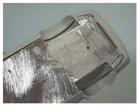
I had to extend the bottom of the rear body inward. I cut a 3-mm styrene tube into several pieces and glue them on the body with super glue.
