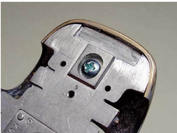
I soldered it to the body and then rounded the edge with a file.
