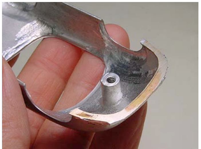
I also removed lots of metal from the inside of the fenders so that the wheels can fit. A sheet of brass at the bottom of the tail will be added to give a clean look.
