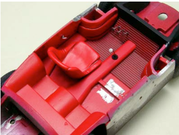
I glued the driver and the passenger seats on the floor. The paint should be removed to for better adhesion.
