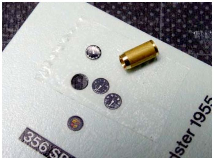
This is an efficient way to make a gauge with glass cover. I put Scotch tape on the decal and punched it with a brass tube.
