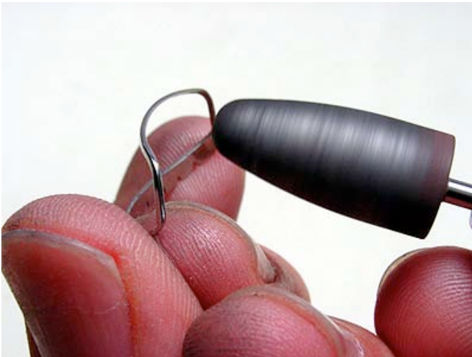
After the soldering I sanded the weld and polished it with motor tool.
