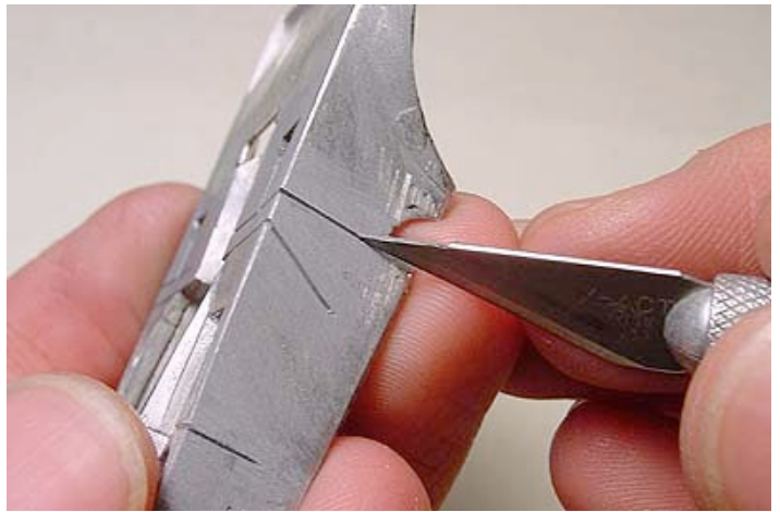
I sanded the surface flat and carved some recessed lines with my X-ACTO knife.(I, as always, painted the surface gray to assess the shape more easily).
