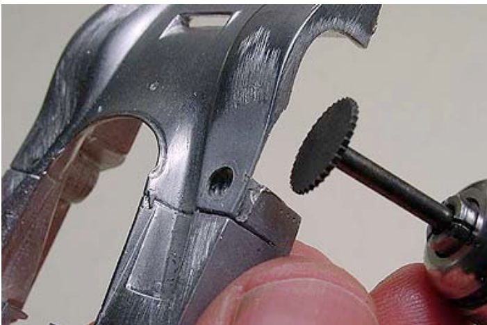
I modified the original fuel filler holes after filling them flat with a solder. And then, to make it look like a very thin racing skin , I began another "surgical operation"!
