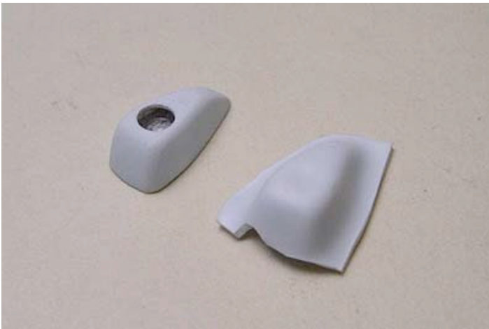
The head-rest included in the kit seems too small for the body, so I added to its volume by vacuum-forming over it.
