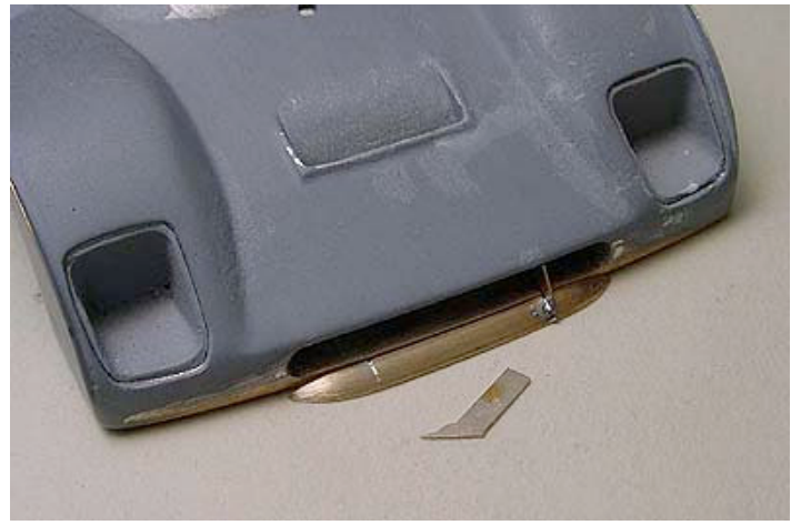
I soldered the splitter plates that were made with 0.2-mm brass sheet to fit in those grooves. The failure is the stepping stone to success; I've got an accurate and sturdy nose-spoiler, finally!
