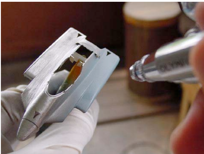
I sprayed the upper cowl with primer. The nose-cone was glued to it temporarily.
