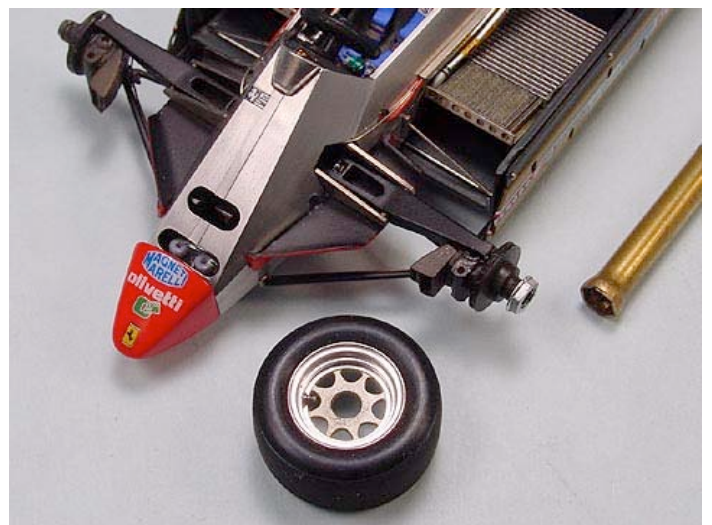
I assembled the front suspension. I also added the stabilizer and steering tie rod.
