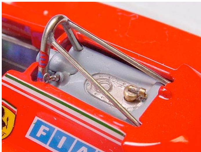
I remade the rollover bar with 0.9-mm and 0.5-mm nickel silver rod. Look at the emergency ignition switch! It was made with a 0.2-mm brass rod.
