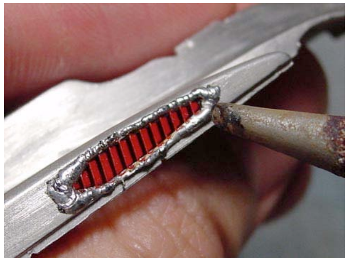
The side air vents are very fine p-e parts, so I soldered them carefully to the upper cowl. It is better I guess, the output of my soldering iron is 25 watts, and the shape of the tip is rather blunt.
