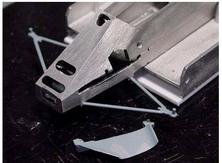
I adjusted the ride height and inserted the 0.75-mm plastic sheet between the under tray and the ground. The upper and lower monocoque were already joined by solder.
