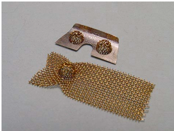
I chopped off the blank space of the mesh. The base plate was made from nickel silver plate.
